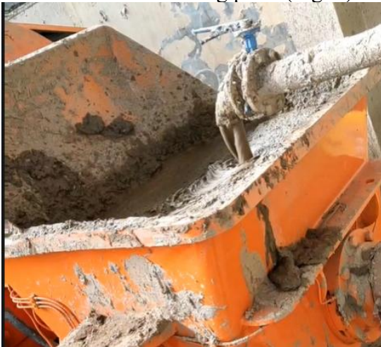
Fig. 2 Circulating pipeline transportation of paste
