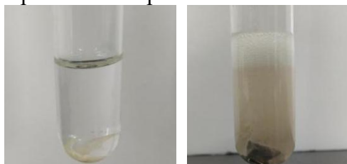
Fig.7 Experiments on nails (left), marble (right) and hydrochloric acid
