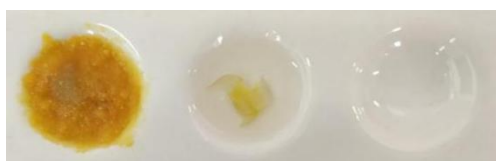
Fig.10 Experiments on the reaction of nails and milk powder with concentrated nitric acid
