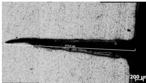
(c) Crack of base metal
