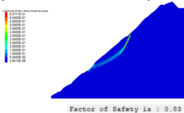
Fig.12 Contour of maximum shear strain increment for natural condition
